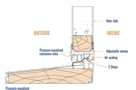
Canada and American Patented door sill system offering the best water tightness and unique pressure balance on the market
